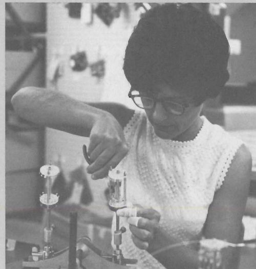
Arlette Fulmer assembles switch for F&M's 5750 gas chromatograph which ranks as one of HP's top selling instruments. F&M products feature complex pneumatic systems often working at high temperatures.
